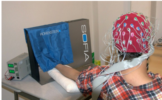
Neurophysiological test subject study using EEG. The textile applicator SOFIA for the first time ever allows textiles to be moved along different parts of the human body with adjustable pressure and adaptable speed. ©Hohenstein Institute – Department of Hygiene, Environment & Medicine
